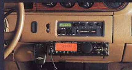
The FT-900AT controls mount almost anywhere in your car, truck or camper. 100 Watt RF deck can mount in trunk, or under seat.
